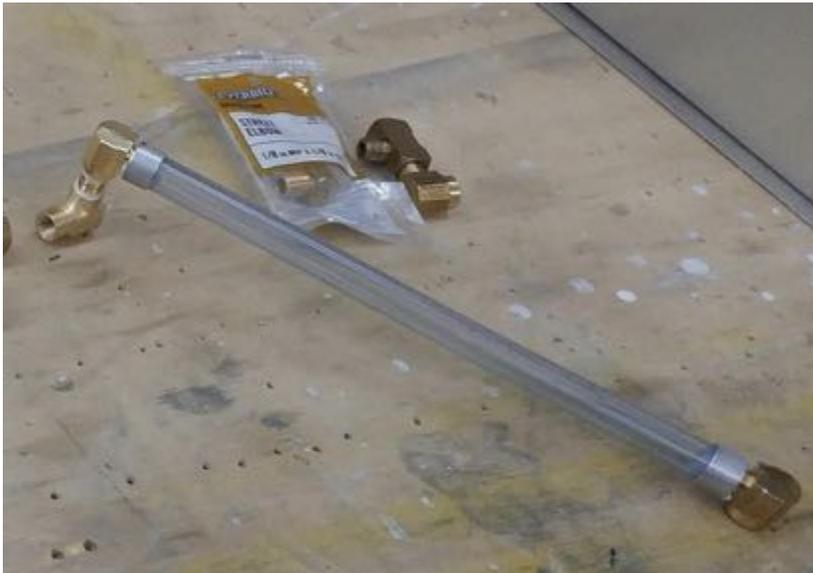
Bushings are pressed over the ends of the sight tube to reinforce the tube and prevent tube expansion in the subsequent operations and over time. The bushings must be a very tight fit on the tube. Bushings are fabricated from 6061-T6 tube, 0.625 OD by 0.035 wall thickness. The bushing ID must be enlarged to fit tightly over the sight tube. A 9/16" drill can be used to ream out the aluminum tube. The bushings are cut to a 1/2" length.
