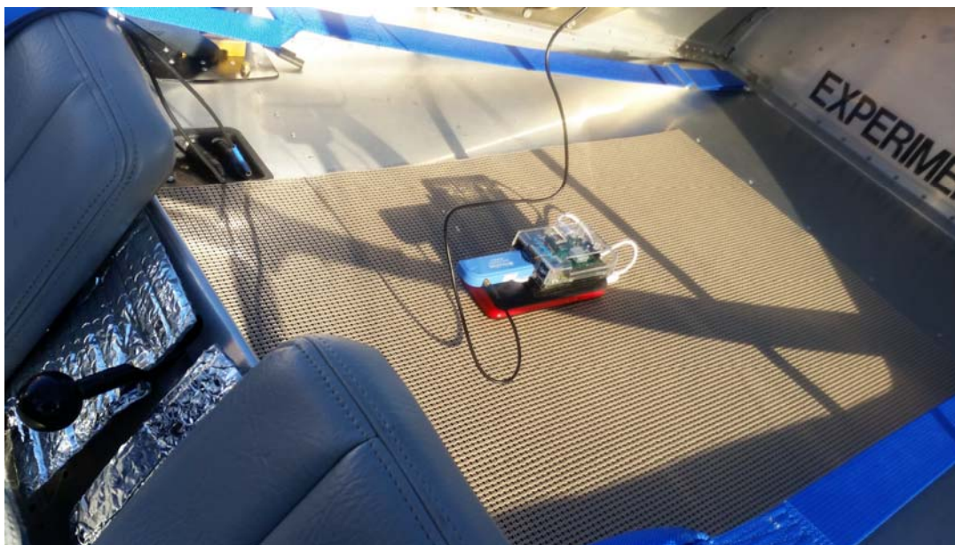
The ADS-B Receiver installed in Pat's Zenith N63PZ for the flight to Texas
