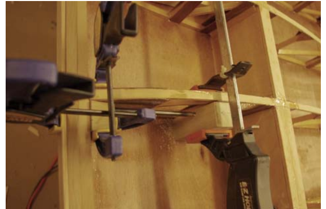
#3—Fitting Rear Support Block
