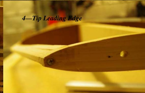
The original plans call for the wing tips to be made of metal, however most builders today make them out of wood. This is the path I chose to follow, which is detailed here.
