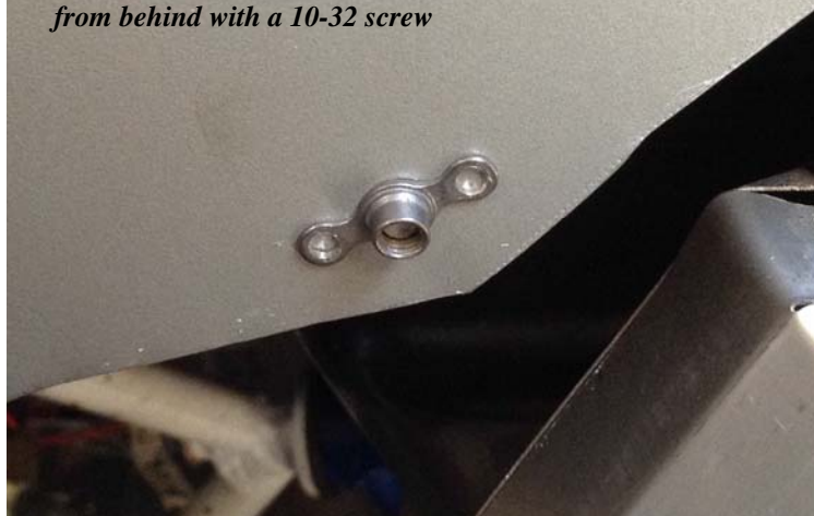
Picture 1—Nut plate held in place from behind with a 10-32 screw
