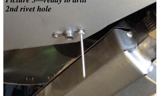
Picture 4—ready to pull the rivets
