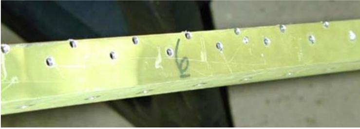
My favorite goof: a buried Cleco deep inside my wing (exactly centered ... 4 feet from either end). I designed a special "long arm" Cleco removal tool. (photo below)
