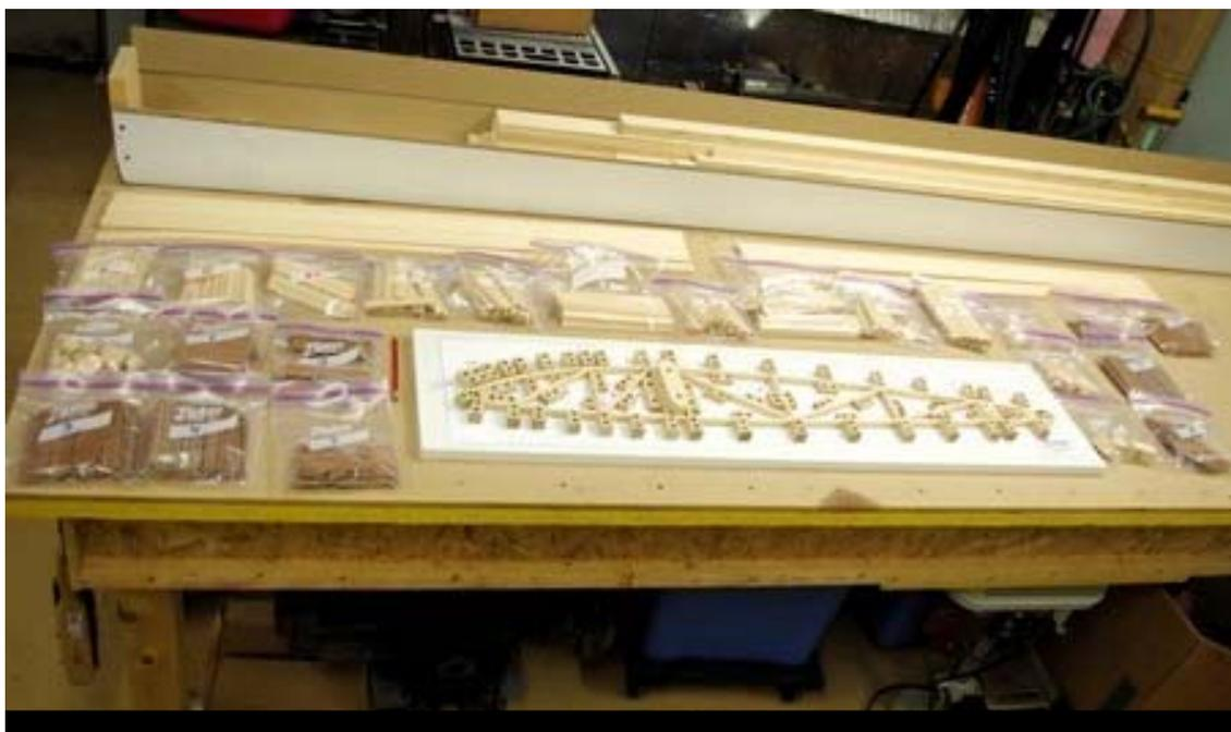
The wing ribs for my current project are made out of spruce and plywood. The main ribs each consist of 14 different pieces of spruce capstrip, 2 different spruce blocks, and 9 plywood gussets of various sizes.
