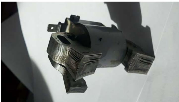
*Damaged magneto coil (impact damage split laminations)*
