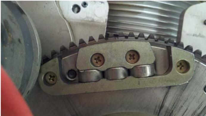
*The flywheel area after repairs with mag cluster attached is functional. The engine is re-installed and two new mag coils are in place. As of November 11th, N167JK is ready to fly again. Thanks for valuable assistance from Bill Brown and Keith Rhode."*
