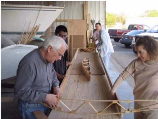
You can see the front and rear spar wood, with the ribs, before building the left wing.
