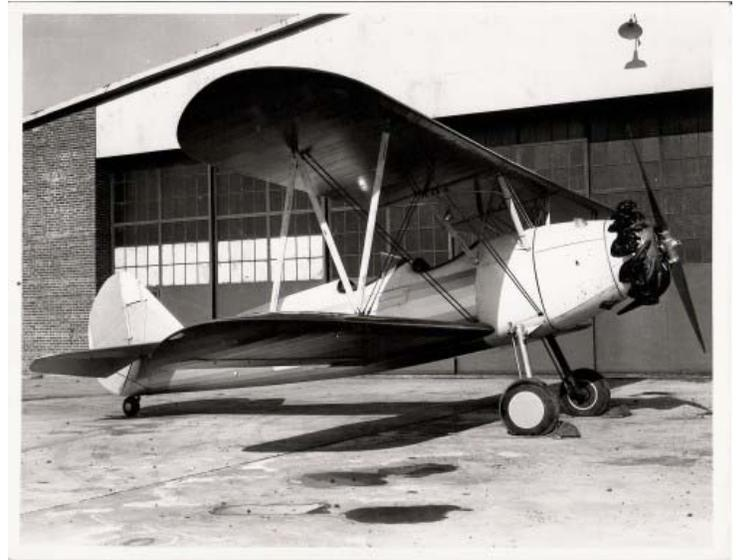
*Above, the 1933 Model 70, with small rudder and unfaired landing gear. The single-leg landing gear did much to distinguish the Model 70 from other open-cockpit biplanes of the era.*
