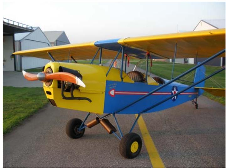
were lengthened and beefed up to stop bending and feet from slipping off during braking. He added cabane hand hold straps, new trim colors, decals and painted the engine cowl and metal boot cowl yellow. We rechecked the weight and balance and the weight turned out to be 732 lbs. That's a little higher than the original paper work. Bungee covers on leading edges were stiffened up for a little better aerodynamics. Aileron gap seals are yet to be installed.
