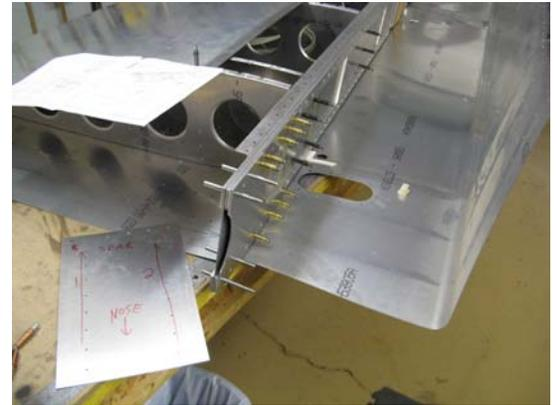
Photo 2—Root Plate and Spar Cap
