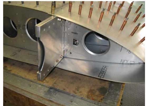
Photo 3—New Spar Plate at Spar Root
