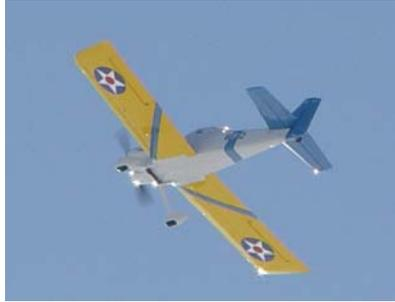
This is Ken's second RV project — he previously built an RV-6A. Ken reports that the new airplane took 1900 hours to construct. Power comes from an O-360-C1G Engine with a Hartzell Blended Airfoil Prop. Empty weight is 1025 lbs, and the paint scheme is from an F-4-F Wildcat from Fighting Six in 1941. You can see construction photos at <http://www.mninter.net/~kbeene/>
