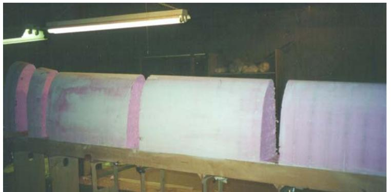
*Fiberglass fuel tanks, now embedded in wings*
