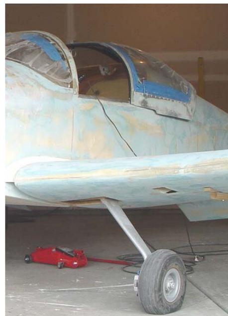
*Note the fixed aluminum landing gear and the fore & aft sliding canopy*
