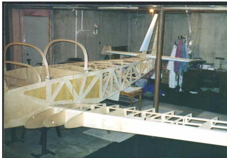
*A wooden airplane with a fiberglass shell—in this photo, you can see the extent of the wood frame in this design, and the high quality of Gary's workmanship.*
