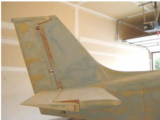
*Gary's new design, without the tail cone, and with the lower fin and rudder*
