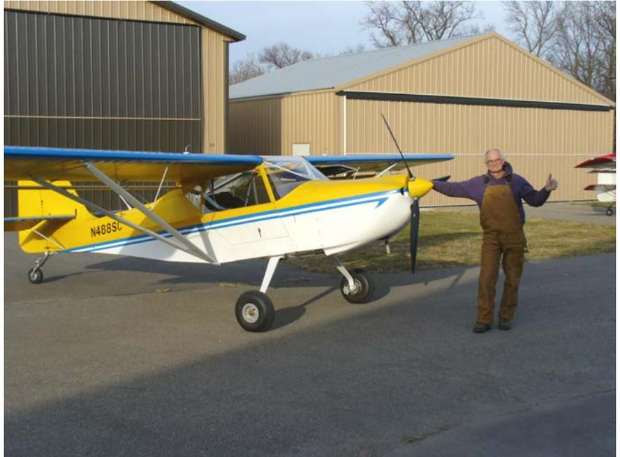
*Experimental Kitfox N488SC completed it's first flight today. Test pilot and fellow Kifox builder Eric Broderson (in the attached picture) reports she flies great...smooth with well balanced controls. The only squawk was that coolant and oil temps were a little low because of the cool weather. I will need to block off part of the radiator and oil cooler.*
