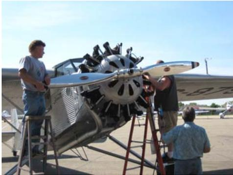
Conducting the compression test on all cylinders
