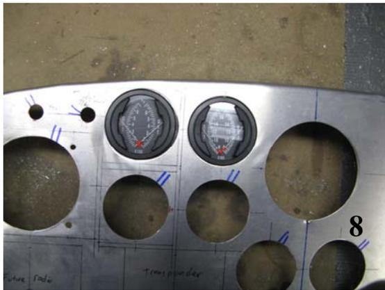
The quality of the holes you can make in your panel is directly related to the quality of the hole saw used. Cheap chinese-manufactured hole saws should be tossed straight into the garbage, as they will have a lot of wobble which will result in larger than expected holes with ragged edges. A good solid hole saw will result in a more precise hole with a smoother edge.
