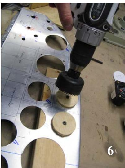
Picture 3 above shows the hole saw with a freshly drilled plywood "plug". I made as many of these plugs as I had instruments of that size, and then I used those plugs as jigs. In pictures 4 and 5 (upper right) a couple of the plug-jigs are screwed down tight into a hole (and into a wooden block behind
