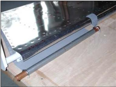
Here’s the last “trick”. The leading edges are hand formed to curved shape and pop-riveted together. Here, you can see how the curve is bent into the otherwise flat skin. This is harder than it looks. I would turn the pipe (fastened with duct tape) with
