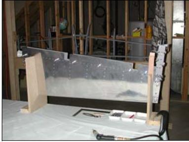
Here is the partially completed right elevator sitting in the “V” jig. You can see the balance arm under construction. Later, a lead weight will be bolted in. The elevators in the RV’s are completely statically balanced (after painting). The
