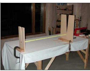
On the left is a picture of the jig used to assemble the rudder and elevators. (The yellow bar across the bottom of the “V” angles is just a tape measure used to get it the right size) Fortunately, the only riveting from this point is by hand squeezer.
