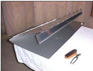
On the left, I have drilled through the right HS skin into the rear spar, temporarily held in place with 9 clecoes. The entire process consists of lining up skins with their corresponding skeleton part and drilling the two together. Later they will align perfectly.
