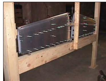
(Did I mention that I tied it into the house structure so it would not move?) I'm told that the "repeat offenders" as Van calls builders of more than one RV, can build the whole tail in the time I took on the jig. I was advised that a couple of two-by-sixes would have been fine. There's no harm in being cautious. Since this would be the first aircraft project I was entirely re-
