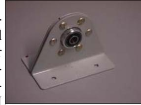
Here’s an outboard elevator hinge bracket. A Heim bearing (rod end) screwed into the moveable surface will connect here. You can see the rear HS spar, two aluminum reinforcing bars, and the steel hinge brackets. Notice the “gold” clecoes. They are for -4 or 1/8 inch rivets. The silver ones above are -3 or 3/32 inch. Aluminum airplane building is a science! BTW, the drill stops are color coded too! The RV uses mainly these two sizes.
