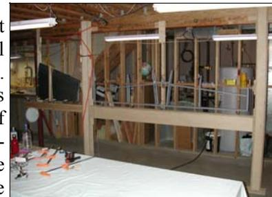
At right is the completed VS, ready for final riveting. After disassembly, each of the holes you see holding a cleco was aligned, drilled, deburred, dimpled (remember, the RV is flush riveted) and re-primed. Then, the whole thing was re-assembled. I think this is the 51% part! The big “C” clamp is just a weight holding tension on a string running across the top of the jig to use as an accurate center line. The plumb-bob is slid along the string to align the parts perfectly.
