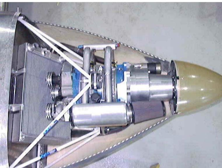
One of the drawbacks of most alternative engines is the RPM's required at full power. In most cases, a big, slow turning propeller is most efficient. The 6000 RPM of the Wankel is far too fast, so a reduction drive is required. One of the most significant features of Powersport's Package is the geared reduction drive (manufactured in house) included with the engine. (They also sell the reduction drive separately.) The Powersport
