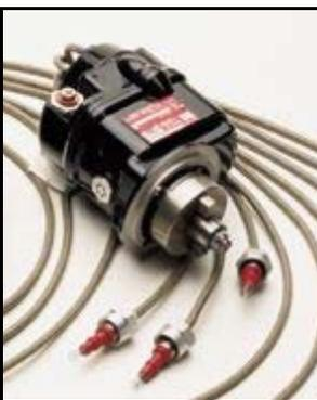
*Magneto and ignition wires: A newer version of the parts that needed replaced on the Cub to improve safety.*
