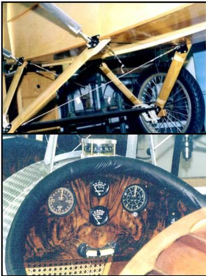
landing gear with tall wire spoked wheels for an authentic antique look. We are not installing brakes and are using a simple tail skid instead of a tailwheel to add to the antique theme but this will limit us to grass strips only.
