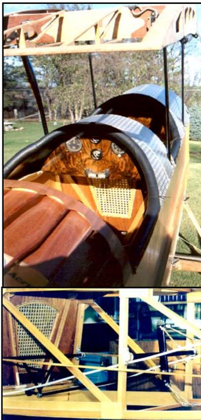
A common theme among Pietenpol builders is to build according to the plans to save weight and keep it authentic. We are staying true to the plans with one exception. The original plans call for cables and pulleys from the control stick to the elevator bellcrank or "walking-beam". There is nothing wrong with this but
